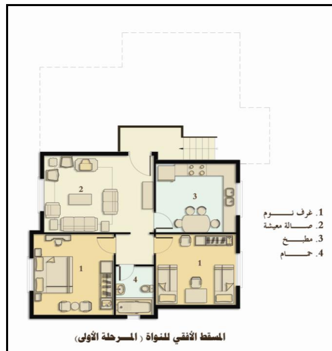
Figure 5.13: The first phase of the Core Unit
